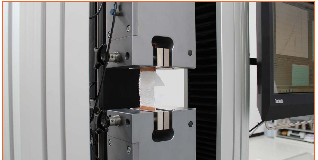
Tensile test on textile, ISO 13934
